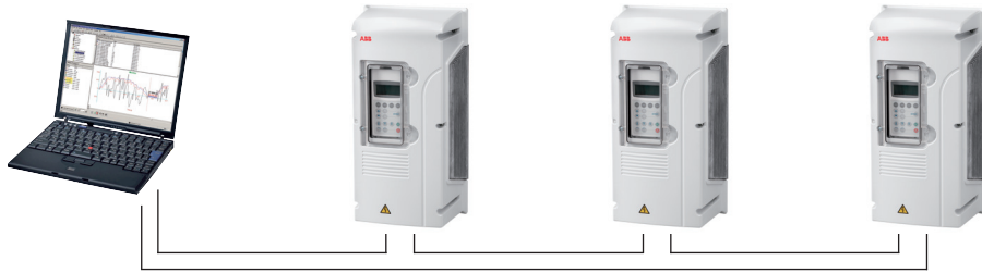
DDCS ring network. PC uses USB or PCMCIA adapter.
