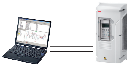
DDCS point to point network. PC uses USB or PCMCIA adapter.
