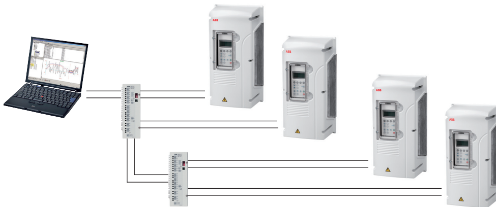
DDCS tree network with optical branching units. PC uses USB or PCMCIA adapter.
