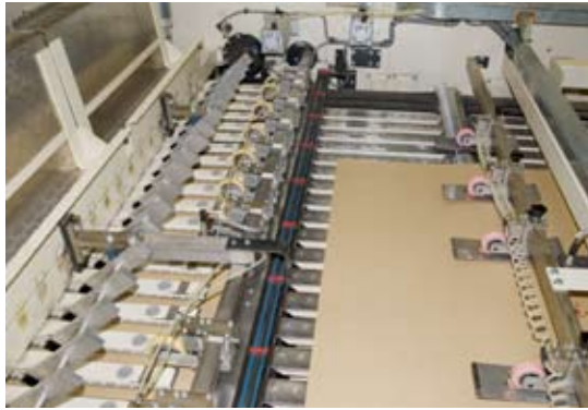
The sheet cutter machine uses the drives to control the rotation of brushes which pushes the cut paper sheets from one conveyor to another.
