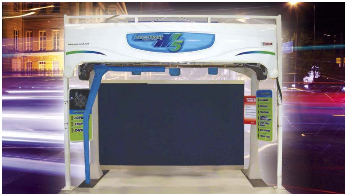
PDQ's new LaserWash M5 is driven by three motors, all of which are controlled by a single ABB machinery drive.
