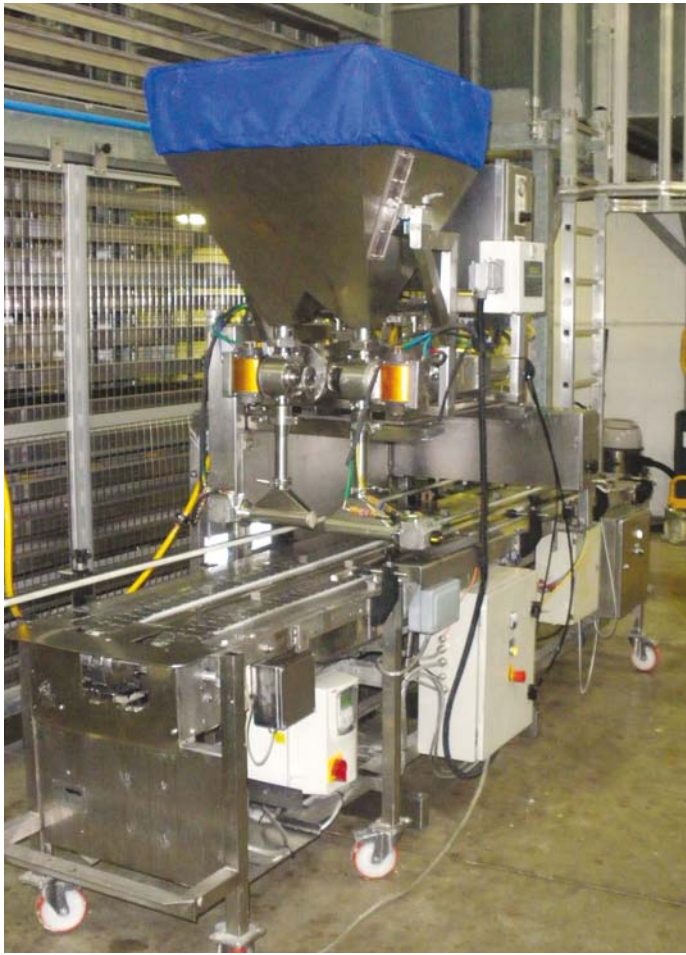
ABB general machinery drive with IP66 protection class allows the bakery to be frequently hosed down.
