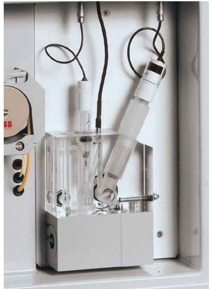
Multi-channel Peristaltic Pump and Sensor Flow Cell
