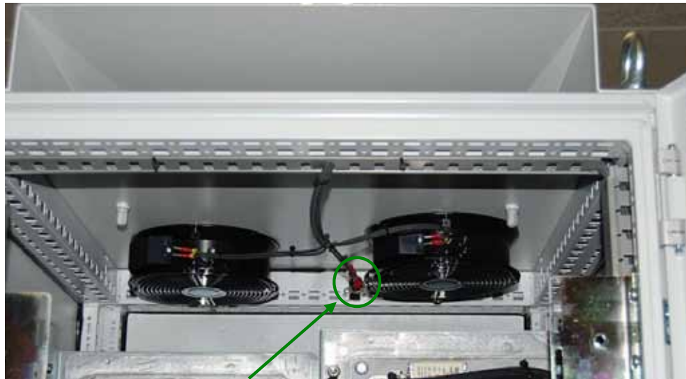
Figure 11: Location of thermal cutoff switch in APCM03 and APCR03
