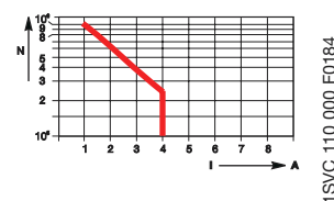
Contact life / number of operations 220 V 50 Hz 1 AC, 360 operations/h
