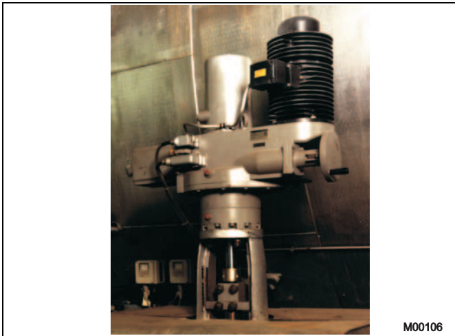
Fig. 35: Linear actuator (feed-water preheating)
