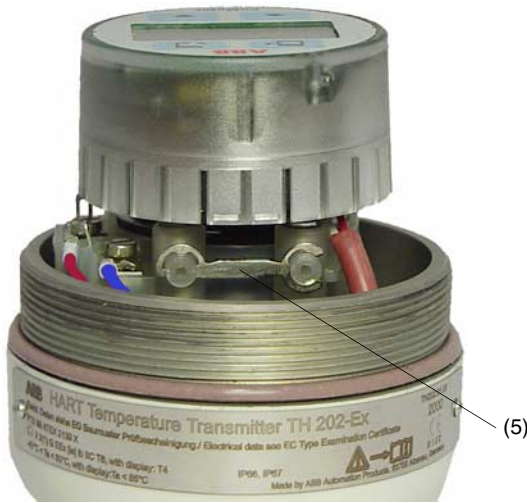
Fig. 4-3 Opened device with indicator (5) Short circuiting bridge in park position without function with devices with indicator
