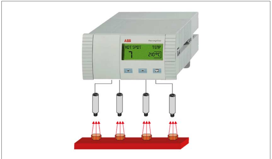
Fig. 2-1 FCU400-IR (SensyCal IR) is designed for monitoring the temperature of power transmission systems
