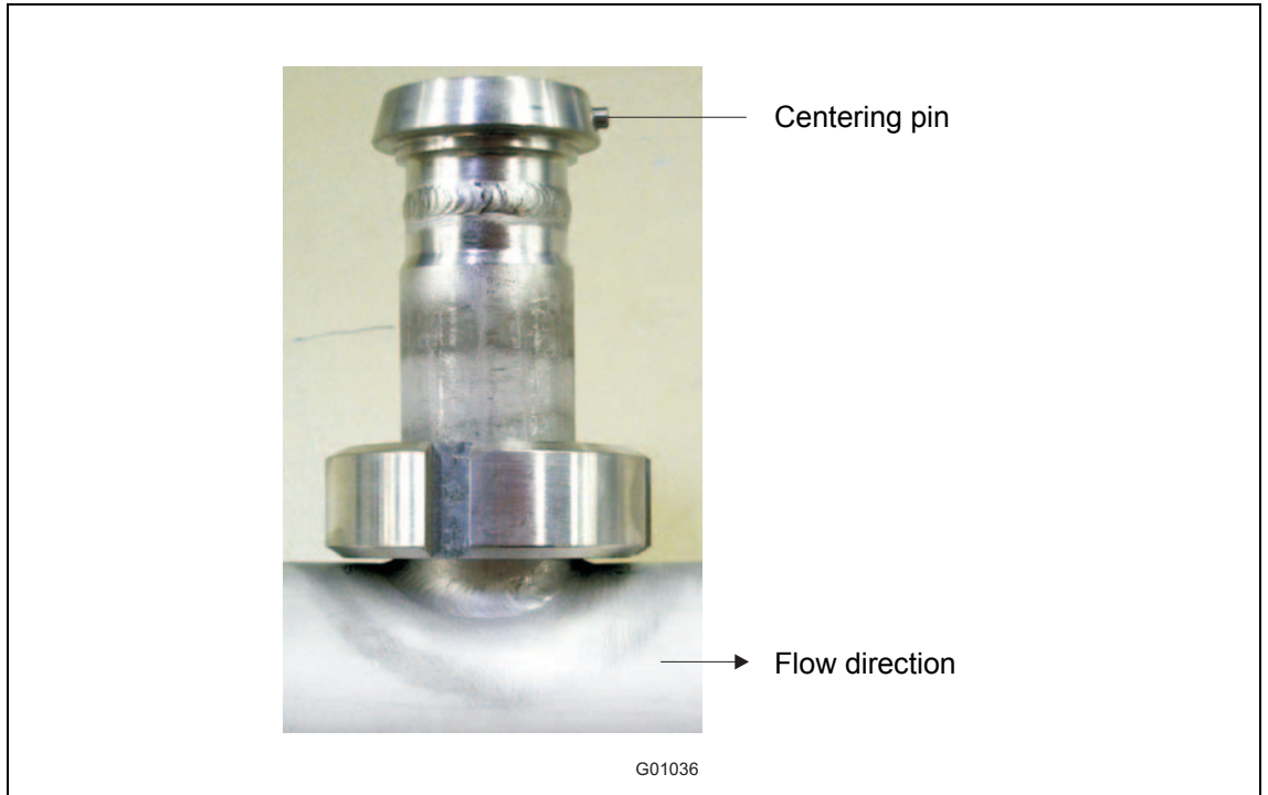
Fig. 5: Weld-on adapter mounted to pipeline, centering pin right (outflow side)
