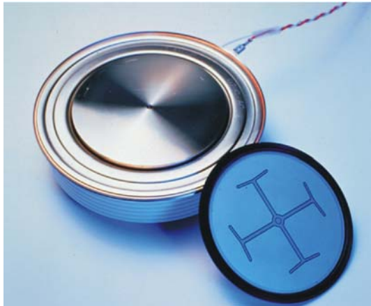
Fig. 1 Modern thyristor with silicon wafer
