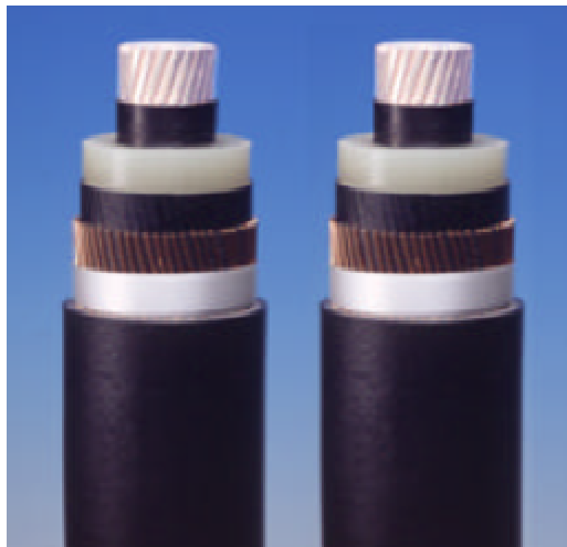
Figure 4. Pair of extruded land DC cables showing from center outward: aluminum conductor, conducting XLPE- layer, dc-insulation XLPE, ground side conductive XLPE, copper shield wires, aluminum outer wrapping and outer sealing and mechanical protection..
