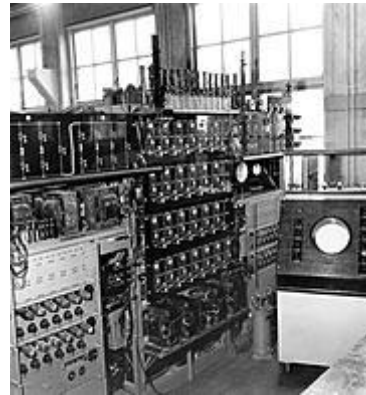
This analog simulator was used in the design of the early HVDC transmissions.
