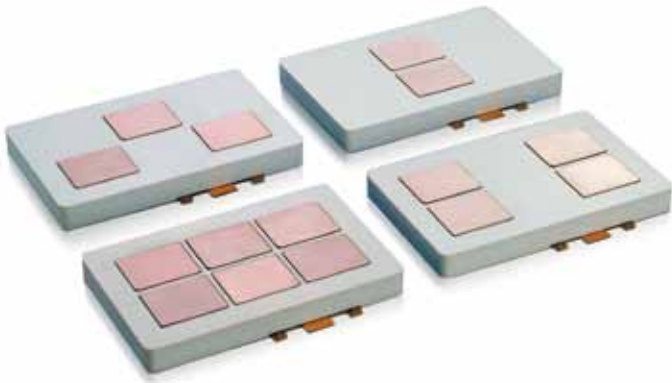
StakPak™ press-pack IGBTs using 2, 3, 4 and 6 sub-modules for different current handling capacity.
