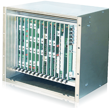
iS3000-19" chassis with integrated CPU
