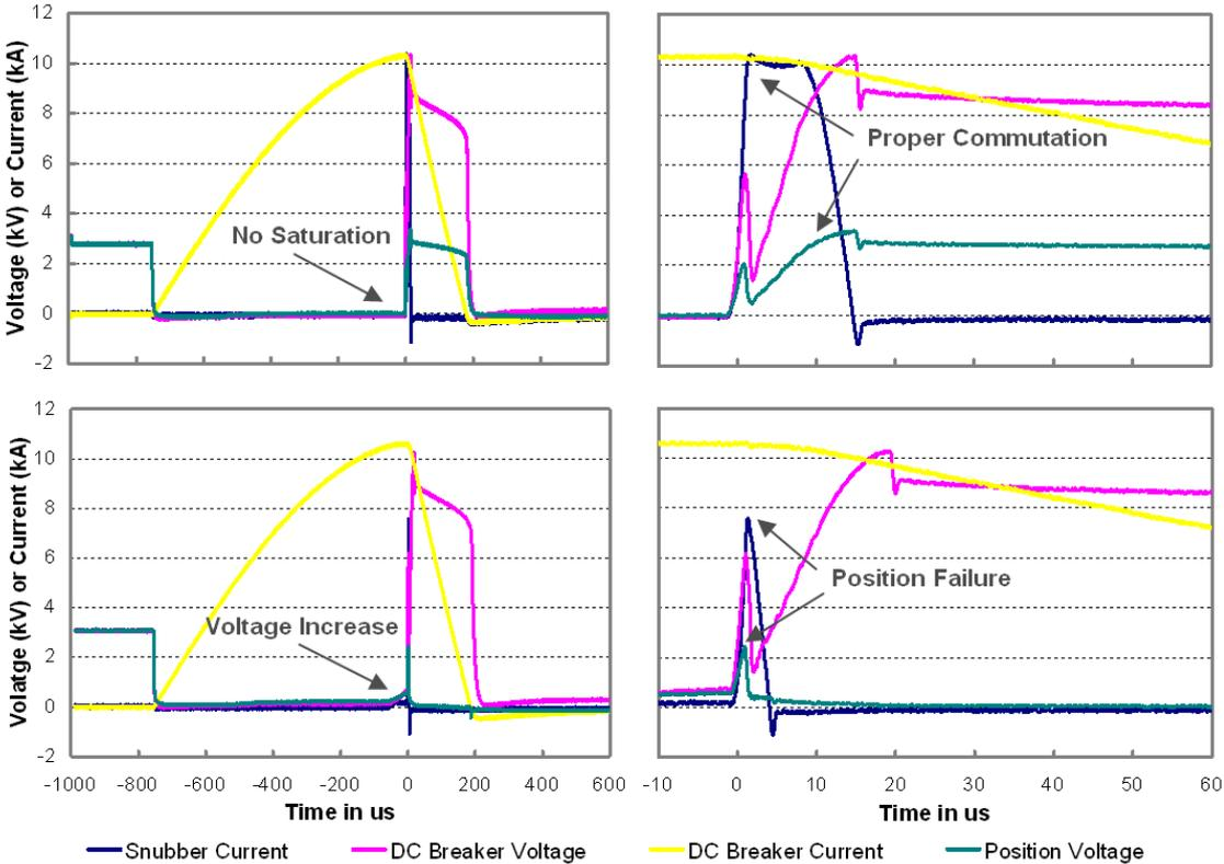
Figure 6: Maximum stress tests on IGBT DC Breaker positions (right: Zoom)
