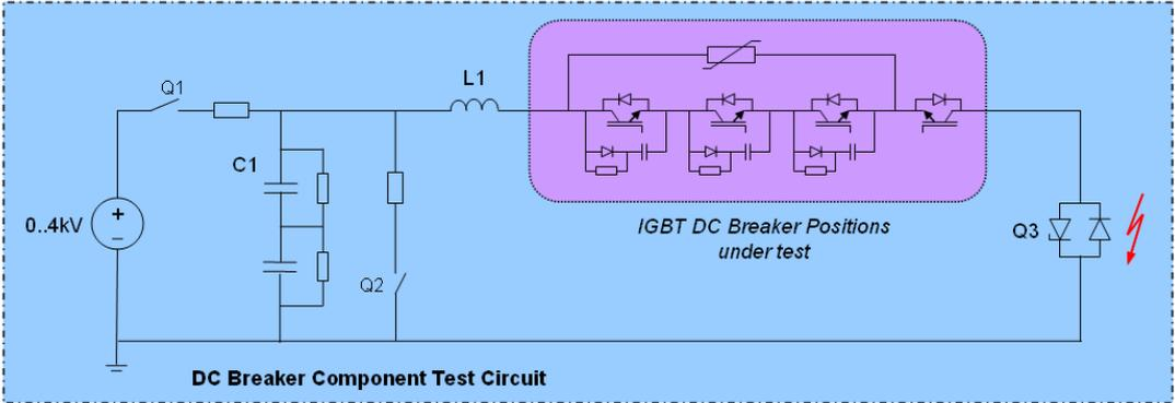
Figure 5: DC Breaker Component Test Circuit
