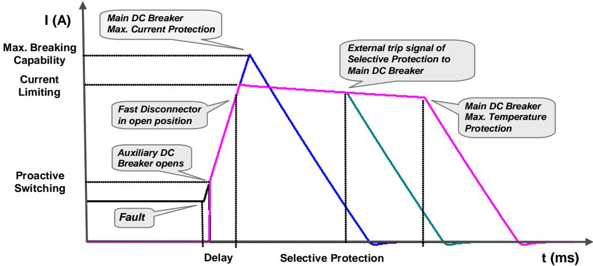
Figure 3: Proactive control of Hybrid DC Breaker
