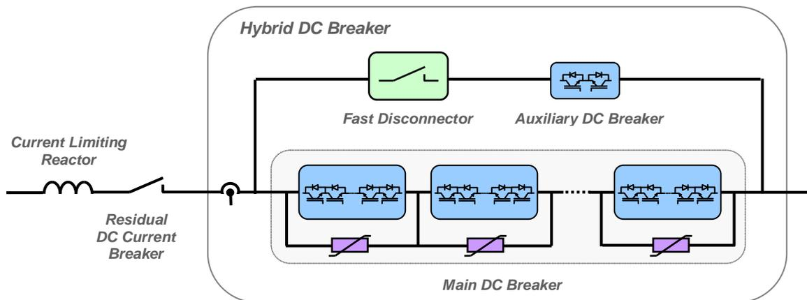
Figure 2: Modular Hybrid IGBT DC Breaker
