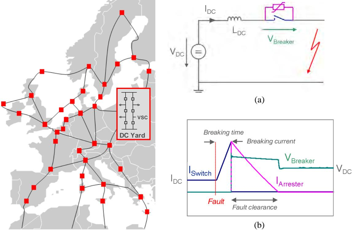
Figure 1: Representation of DC breaker in DC grid
