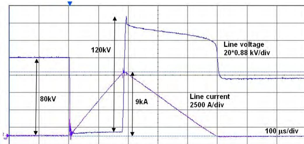
Figure 8: Verification of modular IGBT DC Breaker cell
