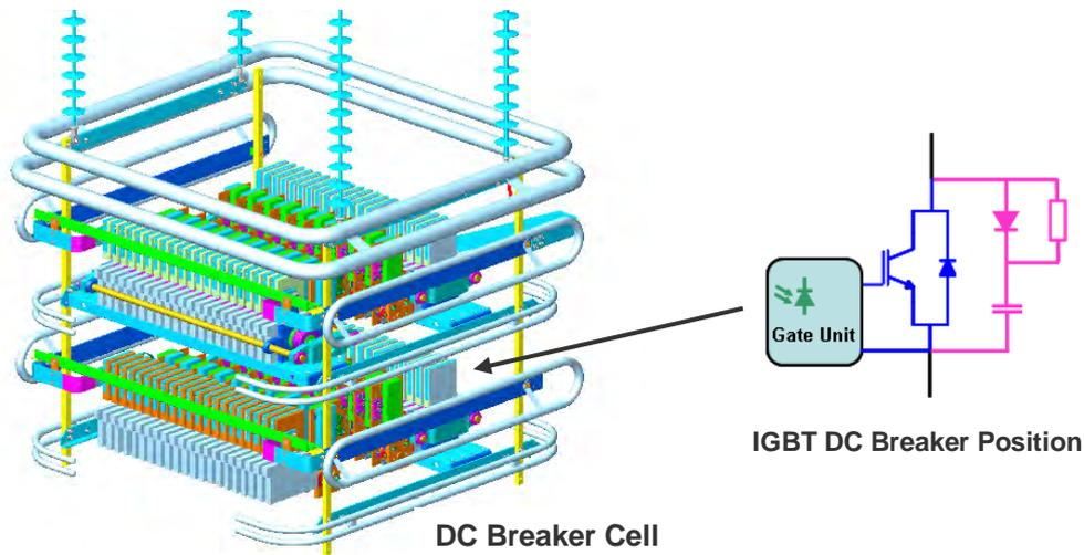
Figure 4: Design of 80kV Main DC Breaker Cell
