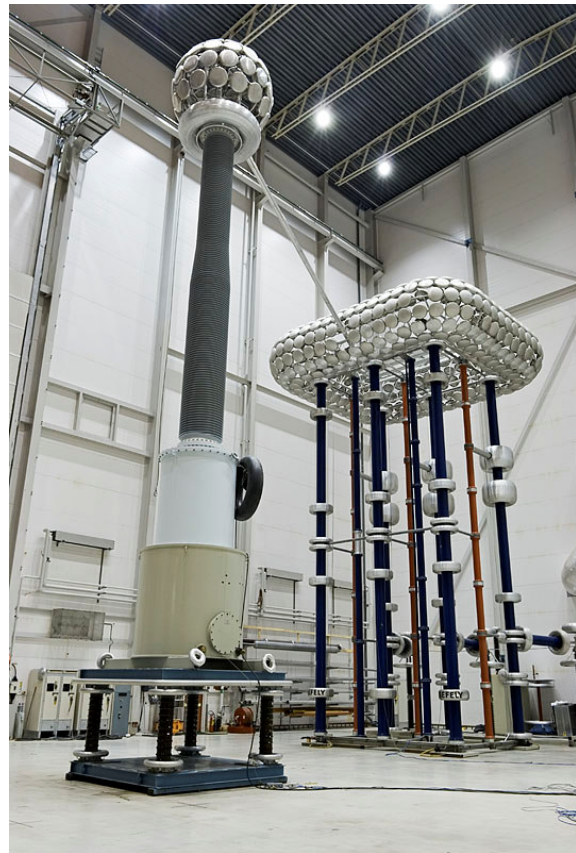
Figure 3: Transformer bushing testing
