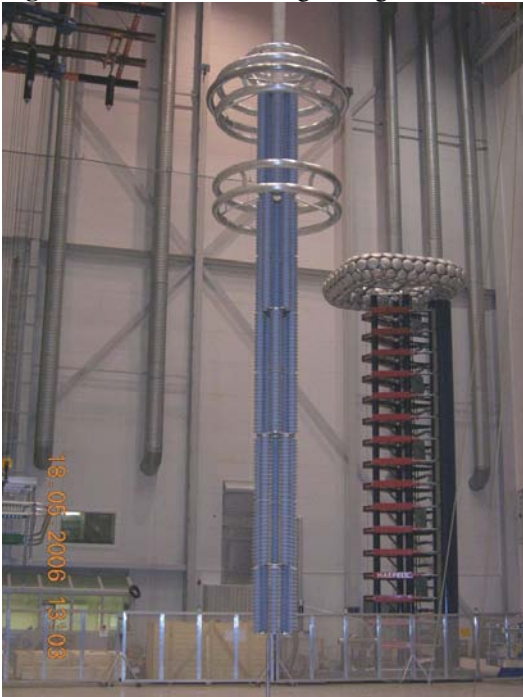
Figure 4: Valve hall bushing testing
