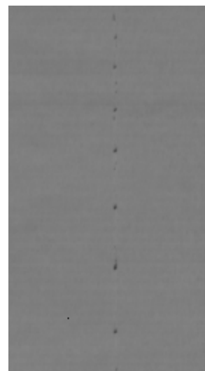
Figure 2 a. Scratch from cold rolling mill
