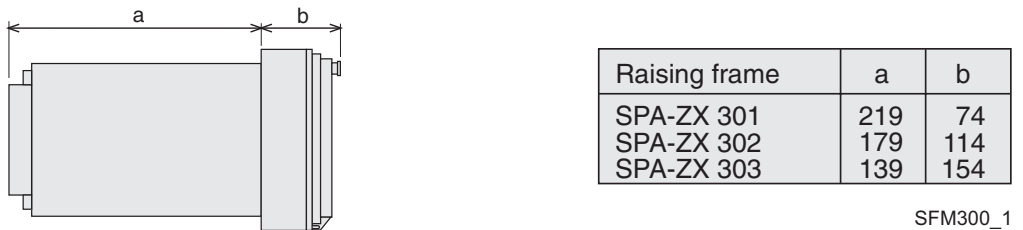
Fig. 3 Semi-flush mounting relay case (dimensions in mm)
