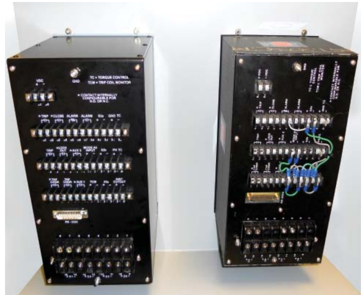
Side by side comparison of the terminal layout of the existing relay and the retrofit assembly.
