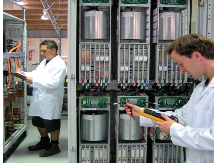
Final quality inspection of an AVC during production
