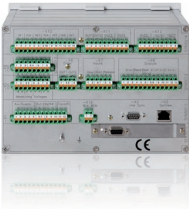
Fig. 10: The conventional connections are made via plug-contact strips. These are largely unnecessary where the communications interface is used; instead, the signals are passed via the 9-pin Sub-D connector at the lower left. The connection to the Ethernet for remote servicing is made via the RJ45 socket.
