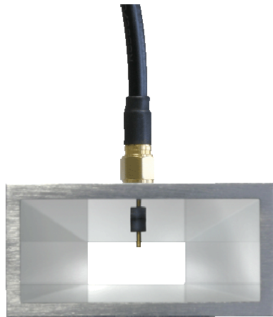
Figure 2. Typical hollow conductor with probe
