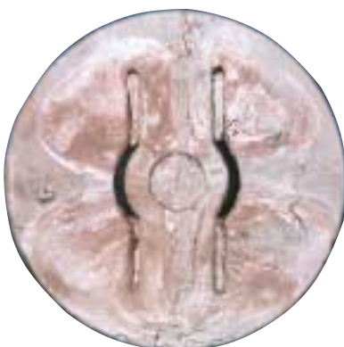
10 Contact surface of a quadrupole contact system after multiple short-circuit current interruptions (63 kA; contact diameter 100 mm)
