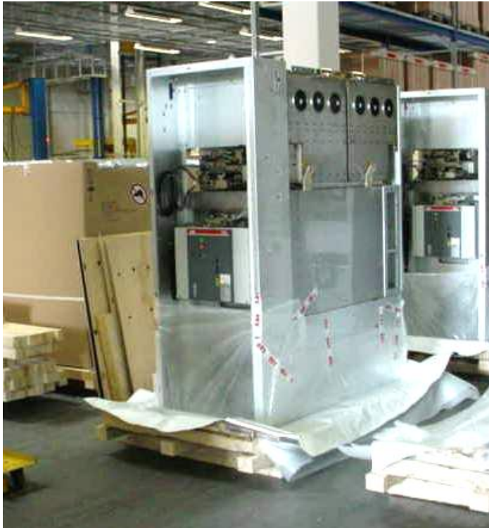
I. Single panel packing gross weight up to approx. 2.5 tons
