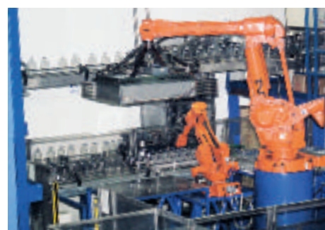
A fully automated sequence where PET bottles arrive at the robot stations by way of the blow-molding machine. 4,000-60,000 bottles per hour are handled and palletized. The full pallets are then shipped to the filling factories.
