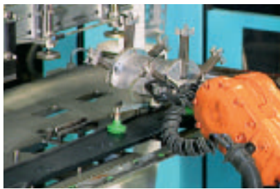
ABB robots are ideal for the assembly of clips onto injection-molded parts. Here the job is carried out on an auto exterior part.
