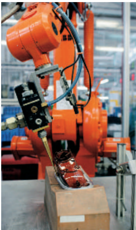
RobotWare Dispense software for gluing and sealing applications speeds up the programming of new parts. Cycle-time and application quality is also optimized.
