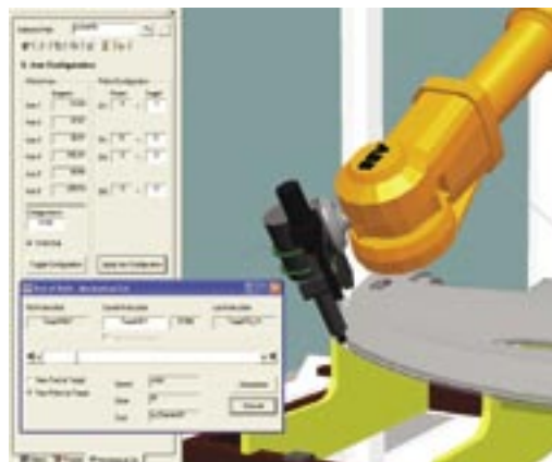
Test your robot programs for potential problems like singularity errors at your desk.
