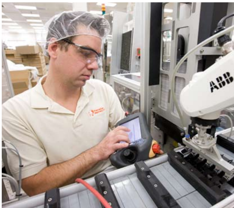
An IRB 120 robot carefully places tubes of INOA hair coloring dye into boxes (left). Sylvain Gauthier (right) of PharmaCos Machinery designed the new installation.
