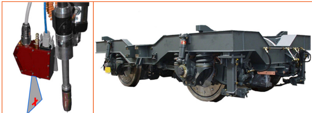
Fig 6: Railway bogie carriage produced using laser scanning sensors
