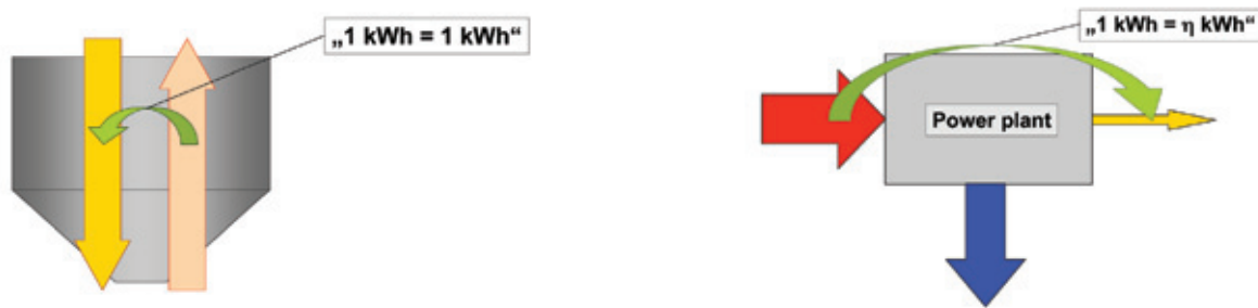
Figure 1. Comparison of waste heat recovery and waste heat conversion. Left: waste heat recovery in a cyclone. Right: waste heat conversion in a power plant.
