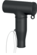
IH-A 24630, IH-A 42630 Insulating sealing hood of flexible rubber with outer conductive layer and an already installed insulating hood. To be installed in HDC-A 630 instead of cable in order to temporarily insulating 630 A switchgear or transformer bushings.
