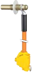
JPB 630 HDC Universal earthing device with two fields of application for 630 A and 12-36 kV: • As earthing-for-work device mounted at the back of a connected cable connector. • As short-circuit protective earthing mounted in front of a disconnected cable connector.
