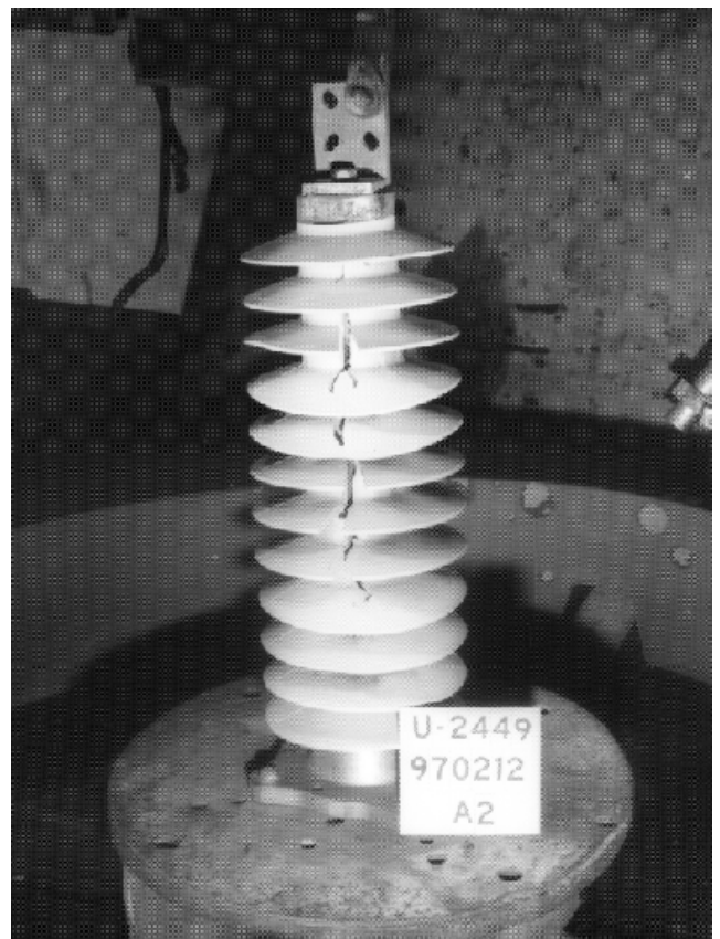
Figure M: The same arrester after a short-circuit test at 50 kA sym
