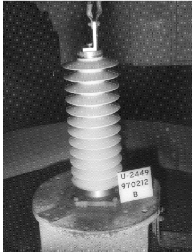
Figure L: A polymer-housed arrester prior to a short-circuit test.
