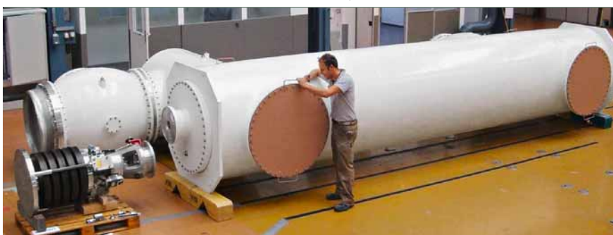
3 The ABB GIS circuit breaker with the drive unit during assembly in the factory
