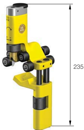
GB-M20 Cutting tool for cable sheath and XLPE-insulation: Diameter: \varnothing 15-50 mm Cutting depth: \leq 8 mm
