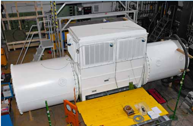
1 A single pole of a heat pipe cooled HECS breaker. From the outside, only the condenser fins are visible on the upper section of the encapsulation
