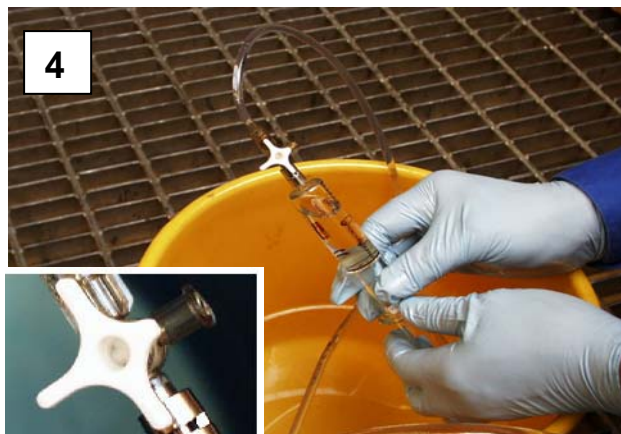
4 Turn the handle of the syringe valve as on the picture. Carefully collect about 20 ml of oil in the syringe.
