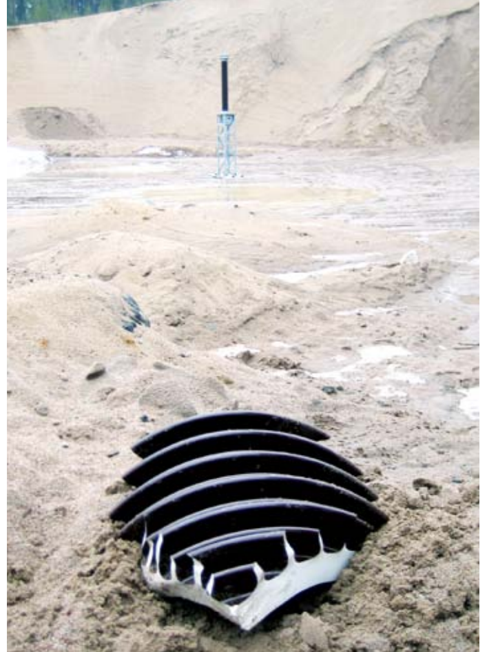
Piece of porcelain insulator after live tank circuit breaker shatter test
