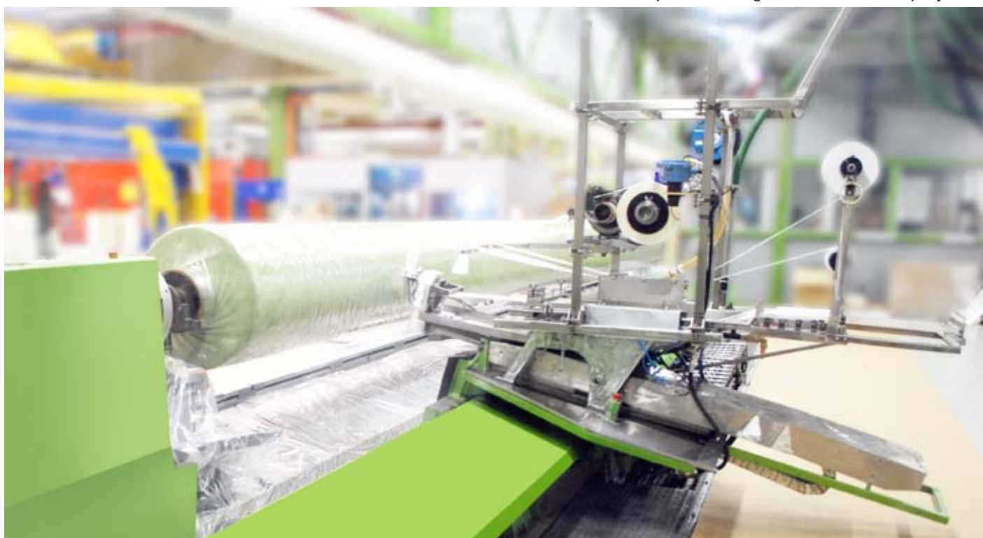
In-house production of glass fiber reinforced epoxy tubes
