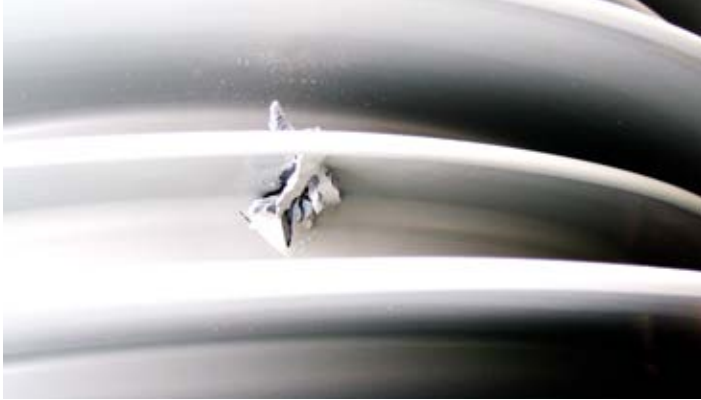
Composite insulator after live tank circuit breaker shatter test
