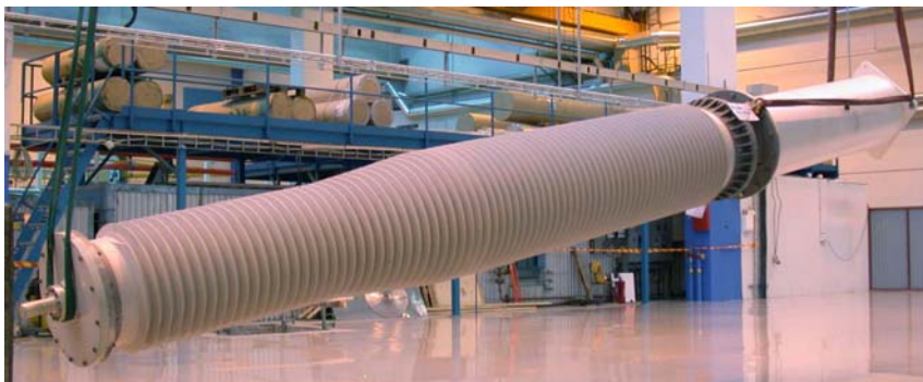
The complete bushing after the test. The high voltage end to the left was at the bottom of the tank and subject to a higher water pressure.
