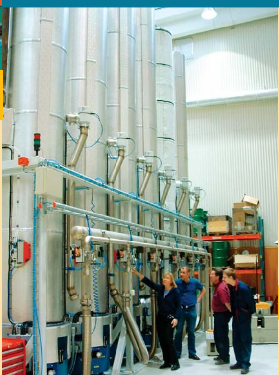
Resin impregnation vessels for RIP bushings up to 550 kV.
