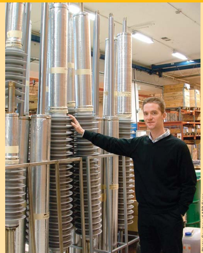
RIP bushings prepared for vacuum processing and injection molding.
