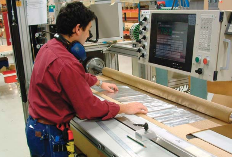
Winding machine for RIP bushing condenser up to 170 kV.
