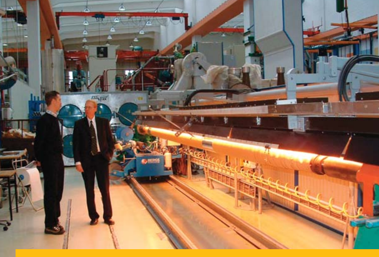
Machine winds condensers up to 12 m in length for use in UHV OIP bushings.
