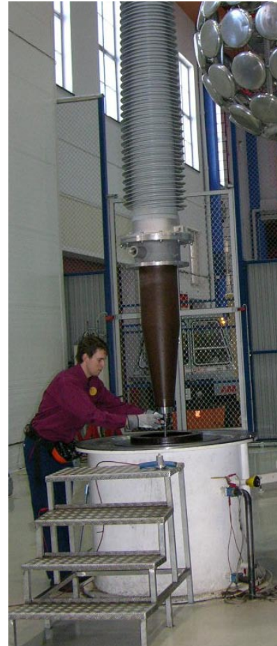
Electrical routine testing of an oil-to-air bushing type GSB.
