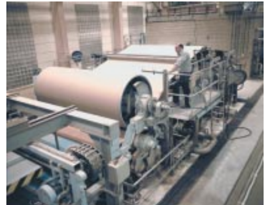
Pressboard production equipment.
