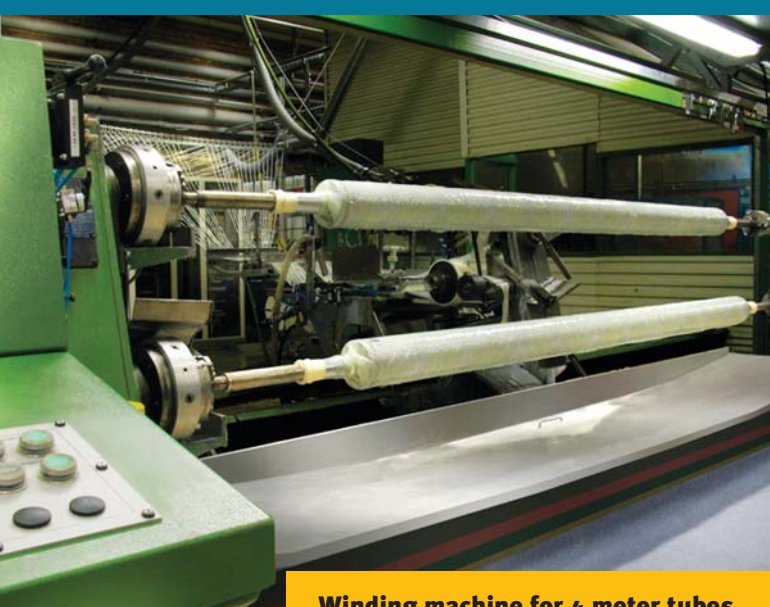
Winding machine for 4 meter tubes.
