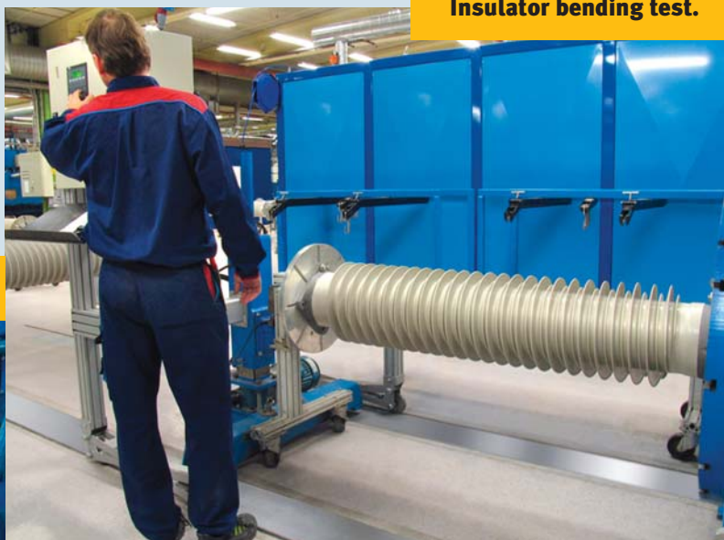
Insulator bending test.
