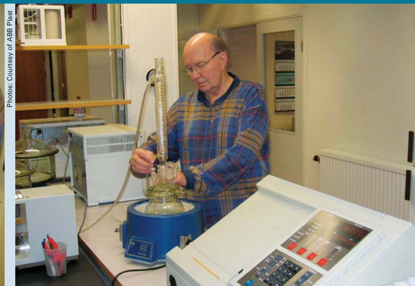
Set-up for IEC boiling test of FRP tube sample.
