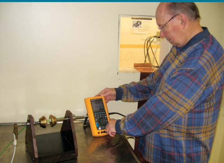
IEC electrical test of FRP tube sample after boiling.
