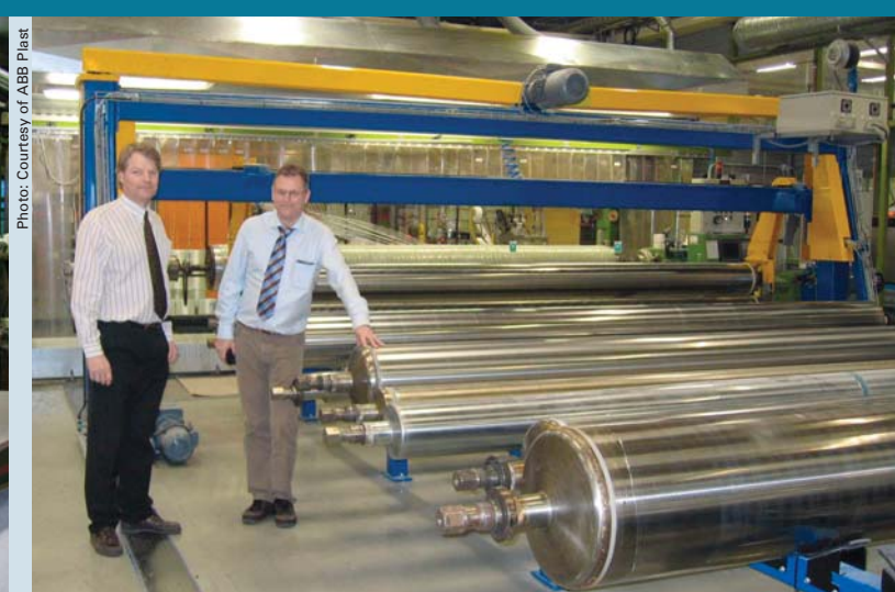
Mandrels for manufacturing FRP tubes (in background stands 7 meter long winding machine)
