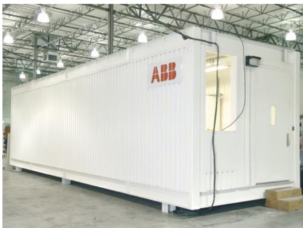
Figure 3. Alagbado Tee building wired for integration testing.
