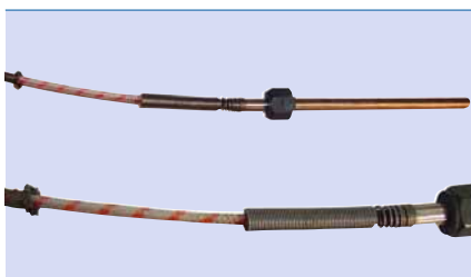
11 Failure in the RTD wire due to high vibration acting on the system
