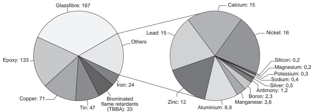
Figure 4. Material content for circuit boards<sup>2</sup>.
