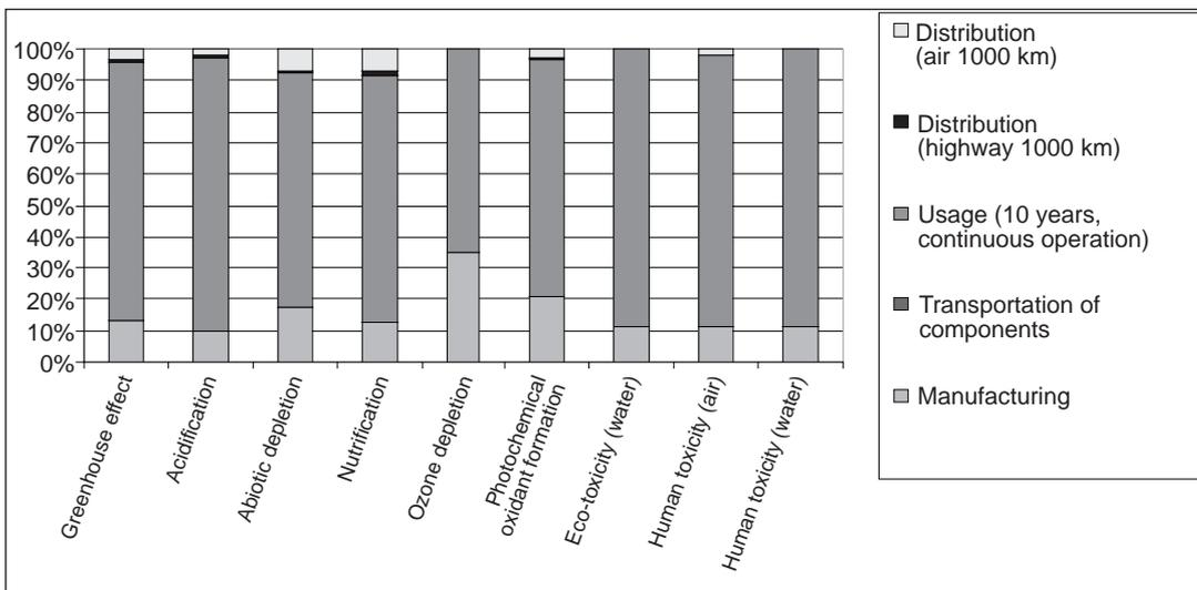
Figure 3. The relative environmental impact for force measurement products.<sup>1</sup>
