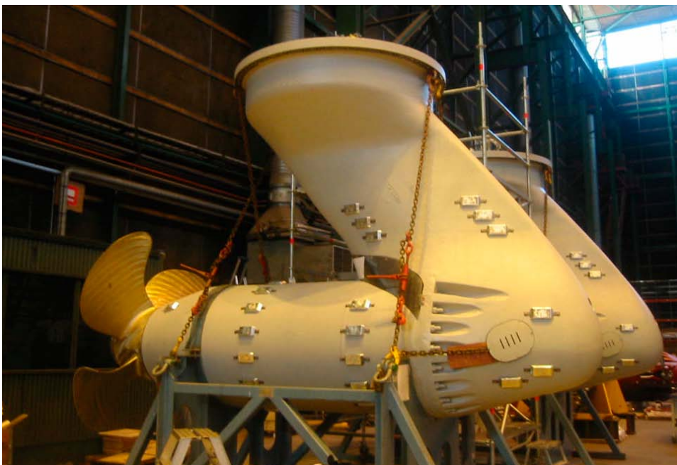
Figure 5-7 CO steering propulsors for “Ice” ready for dispatch to the Lürssen shipyard
