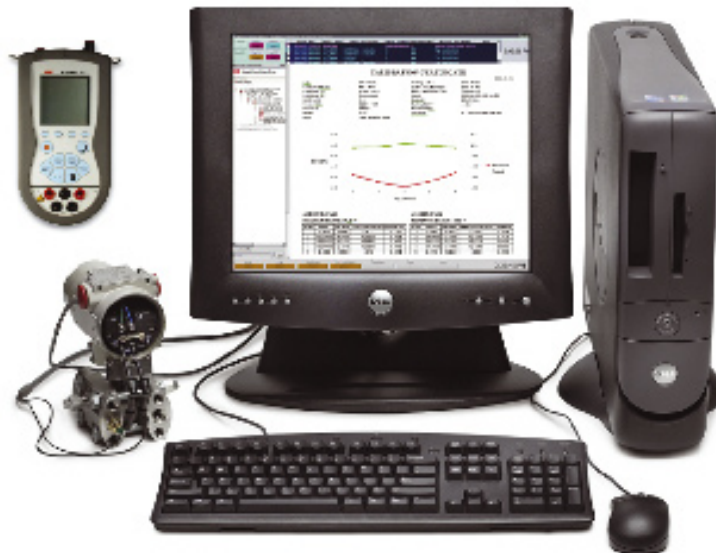
Figure 11. DMS Calibration Software connectivity to 800xA Fieldbus Management Tools
