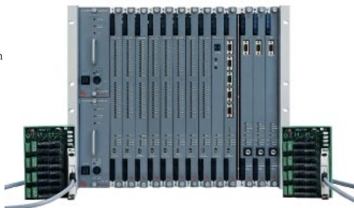
Triguard SC300E Chassis System plus cables and Termination Modules
