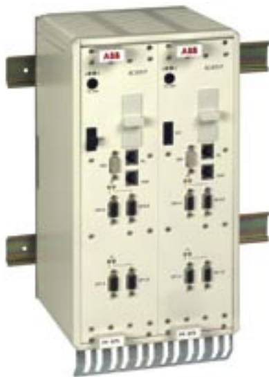
Figure 3: PH 875 housing with redundant PM 875 controller
